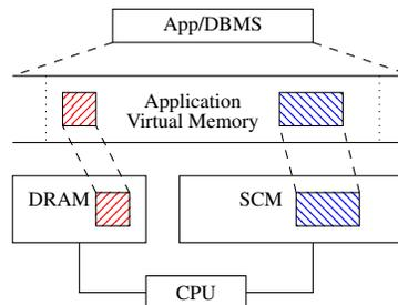
**Figure 2: SCM is mapped directly in the address space of the application.**
