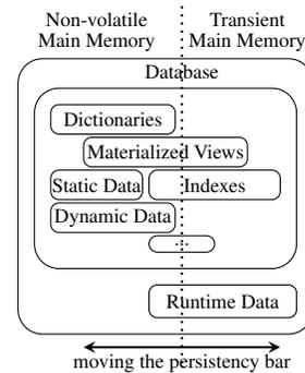
**Figure 4: SCM-Enabled database architecture.**
